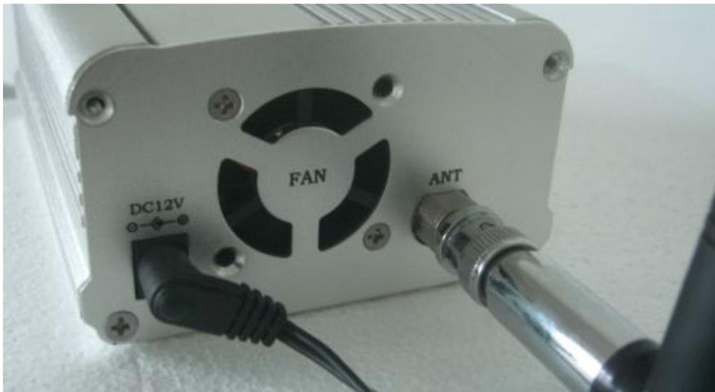
In the back of the transmitter, the antenna interface (ANT) as a BNC interface, therefore, the antenna interface should also be as BNC. External power adapter output voltage DC10 ~ 14V should be within the range of maximum output current should be in 4A above. As shown, the power adapter DC plug connected to the transmitter back "DC12V" on top
